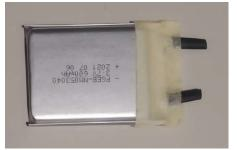
comes close to the board (in particular to the charger connectors) it can get cut and damaged. To prevent this and to hold the battery tight, spacers are applied to the battery, as in figure. The spacers between the battery and the board are placed as the 2 pictures showed below.
