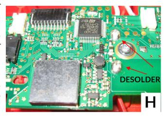
board gets disconnected. This is a good time the make sure the charge connectors do not have sharp points that might damage the battery. In case make them round with a small iron file.
